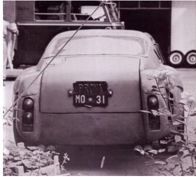
Description: Cut off back with thick side fins
